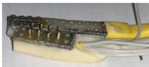
Figure 1. Sensors developed. Left – For assessing setting process of concrete mixes, Right – For detecting water penetration through the concrete surface.
