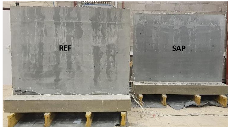
Figure 1: Large scale testing walls, on the left is the reference HPC mixture wall (REF) and on the right HPC wall with SAPs
