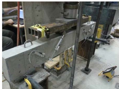
Figure 1: Reinforced ECC beam specimens under flexural loading
