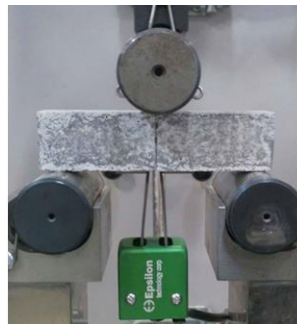
Figure 2. Controlled damage of prismatic specimen
