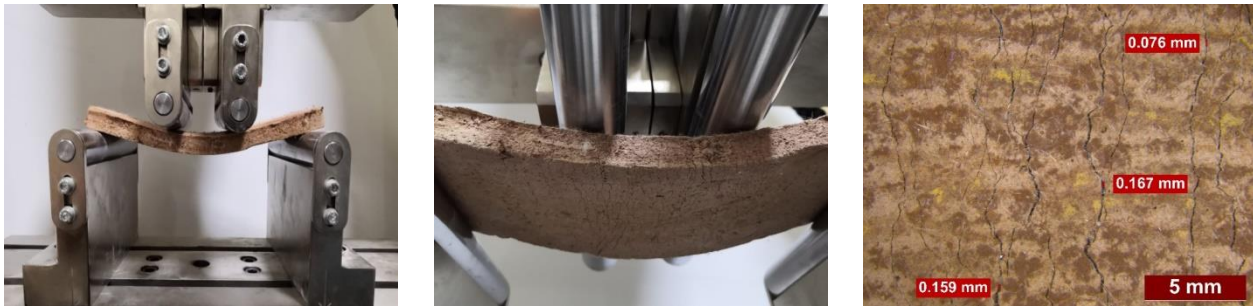
Figure 1: Representative views of EGC specimens and microcracks after bending test
