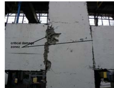
Spatial model of the hybrid joint: overall testing assembly
