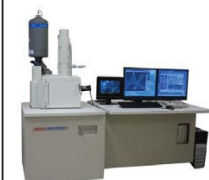
Scanning Electron Microscope with Energy Dispersive Spectroscopy – JEOL JSM 6460 LV, Oxford INCA
