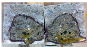
Studying the flow of healing agents in cracks
