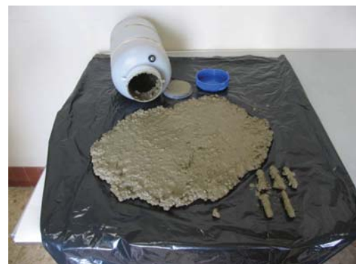
► Cementitious hollow tubes survived mixing...
