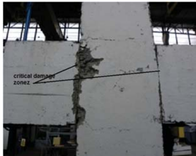
Planar model: critical damage areas after testing
