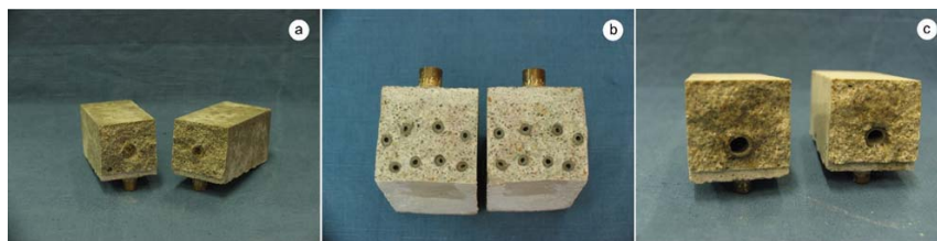
► Prisms for 3-point bending tests w cementitious hollow tubes
