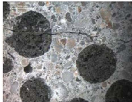
Expanded clay particles impregnated with bacterial spores and calcium lactate and (Jonkers, 2010)
