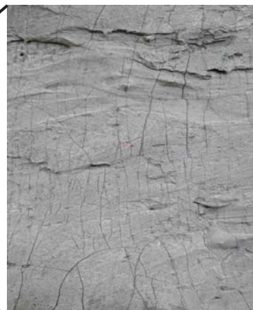
PVA fabric impregnated in cementitious matrix
