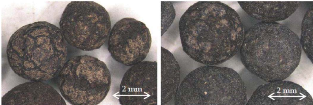
Encapsulated lightweight aggregates (clay) before and after (Sisomphon et al, 2011)
