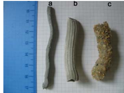
► Cementitious hollow tubes w/o and w final coating
