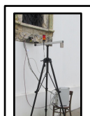
X-Ray Fluorescence Spectrometer – Bruker Artax µXRF 200
