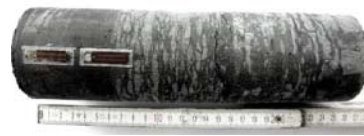
Strain-hardening cement-based composite after a short-time dynamic tension test
