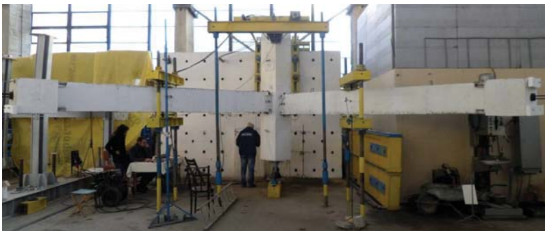
Planar model of the hybrid joint: critical damage areas after testing
